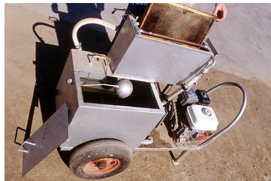
Close-up of machine used to spray syrup into combs.
