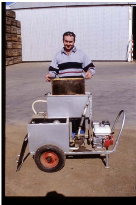
Ken demonstrating machine built to spray syrup into combs.
